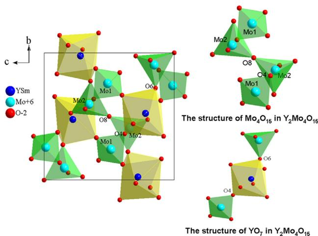
Fig. 1.  $Y_2Mo_4O_{15}$  cells and the coordination environments therein (the blue balls are yttrium atoms, the red ones are oxygen atoms, and the turquoise ones are Mo atoms). (For interpretation of the references to color in this figure legend, the reader is referred to the web version of this article.)
