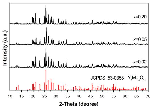
Fig. 2. XRD patterns of three representative  $Y_{2-x}Mo_4O_{15}:xSm^{3+}$  samples ( $x=0.02, 0.05,$  and  $0.20$ ).
