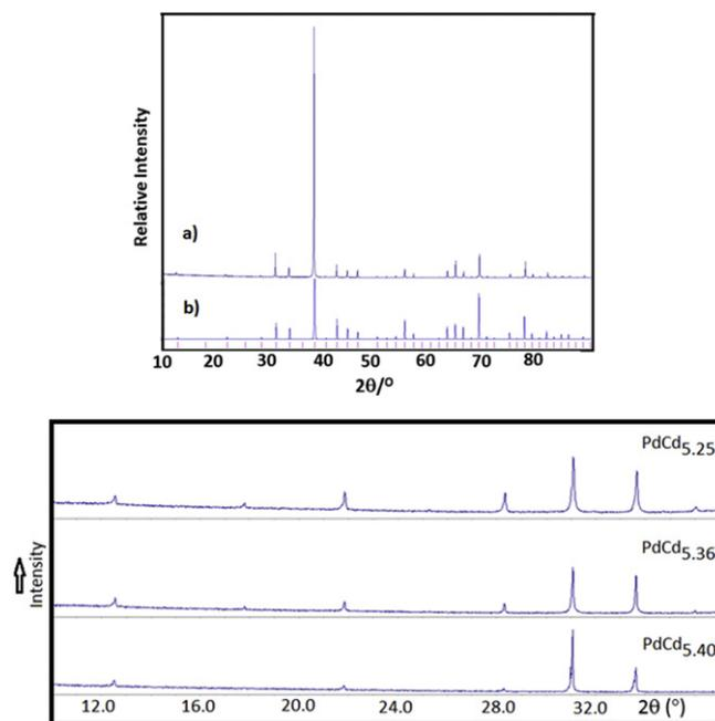
Fig. 1. (top) Experimental (a) and calculated (b) X-ray powder diffraction pattern of  $\gamma$ -brass type  $\text{Pd}_2\text{Cd}_{10.79}$ . Vertical bars indicate the corresponding Bragg positions. (bottom) X-ray powder diffraction patterns in the  $2\theta$  range  $10^\circ$ – $37^\circ$  observed for single phase samples  $\text{Pd}_2\text{Cd}_{10.49}$ ,  $\text{Pd}_2\text{Cd}_{10.72}$ ,  $\text{Pd}_2\text{Cd}_{10.79}$ .
