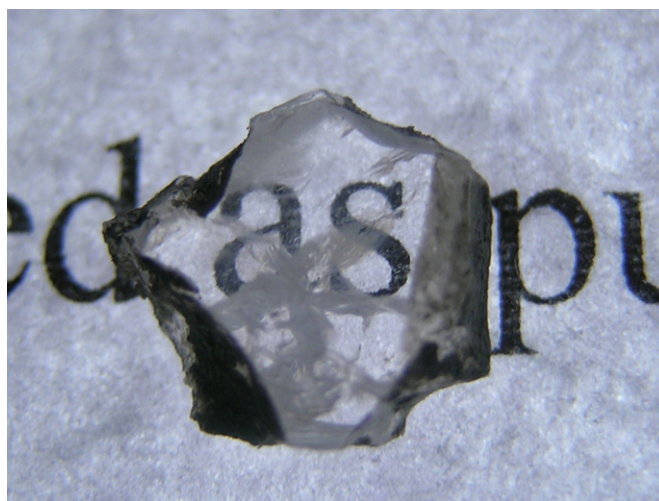
Fig. 1. Photo of K_3WO_3F_3 single crystal on the background of Times Roman font 12.
