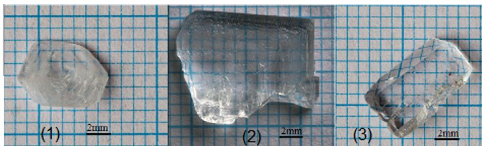
Fig. 1. Photographs of (1) lead(II), (2) mercury(II) and (3) strontium(II) methanesulfonate crystals.
