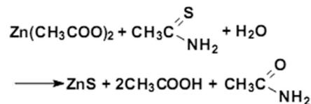
The  $\text{Zn}_{0.998-y}\text{S} : \text{Ce}_{0.001}\text{Li}_{0.001}\text{Mn}_{(0.001 \leq y \leq 0.03)}$  nanophosphors were synthesized via the above mentioned method by using (2.1883 g ( $y = 0.001$  mol), 2.1685 g ( $y = 0.01$  mol), 2.1246 g ( $y = 0.03$  mol)) of zinc acetate, 0.7513 g of thioacetamide, 0.0031 g of cerium acetate, 0.0010 g of lithium acetate and (0.0024 g ( $y = 0.001$  mol), 0.0245 g ( $y = 0.01$  mol), 0.0735 g ( $y = 0.03$  mol)) of manganese acetate respectively.
