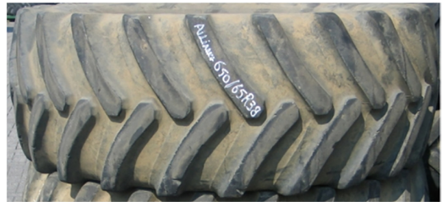
Fig. 1. Side view of AGRI-STAR R-1 W tire.
