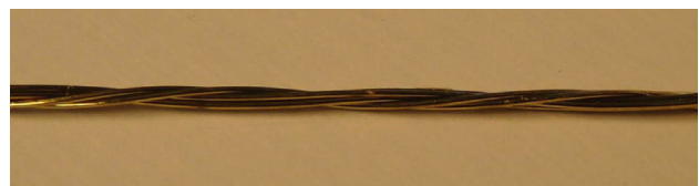
Fig. 1. Steel cord manufactured with five wires.
