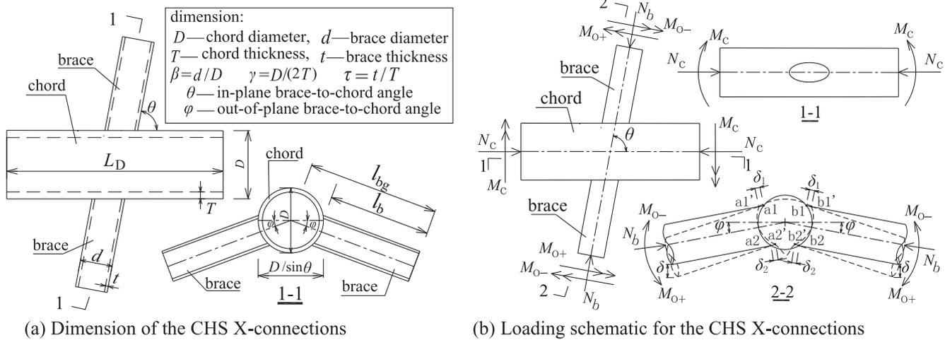
Fig. 1. Geometric parameters and loading diagram of multi-planar CHS X-connections.
