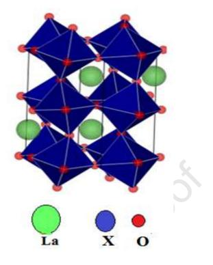
Fig.1: Structure for LaXO<sub>3</sub>(X= Cr, Mn, Fe) in orthorhombic phase 62-Pbnm.
