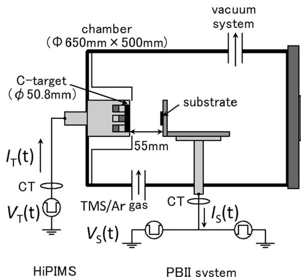
Fig. 1. Illustration of HiPIMS combined with PBII system.
