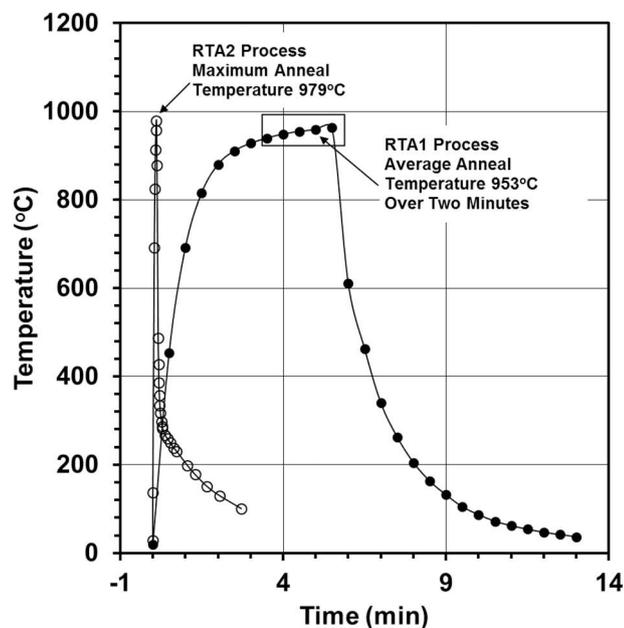
Fig. 1. Typical temperature vs time profiles for RTA1 and RTA2 annealing processes. This illustrates the marked difference in heating rates. For the RTA1 process, the rectangular insert corresponds to the portion of the profile associated with the anneal.
