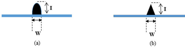
Fig. 1. The Schematic shape of the bumps on the surface (a) Elliptical bump (b) Triangular bump.
