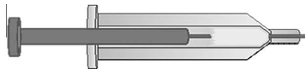
Fig. 1. Schematic of the syringe used to extrude collagen conduits. The diameter of the inner rod dictates the inner diameter of the collagen tubes, which is 1 mm. The annulus region, through which the collagen is extruded, has a thickness of 0.5 mm and the length of the cylindrical cavity is 7.5 cm. 0.1 ml of ~30 mg ml -1 collagen solution is injected into the hollow cavity of the syringe. The inner rod, which is 5 cm long, is then manually forced through the annulus, extruding the collagen at a volumetric flow rate of 0.124 cm 3 s -1 . The extrusion process coats the inner rod with a 0.5 mm layer of collagen, which is then immediately soaked in 10× PBS at 37 °C for 5 min to initiate fibril formation and stabilize the collagen fibril alignment.
