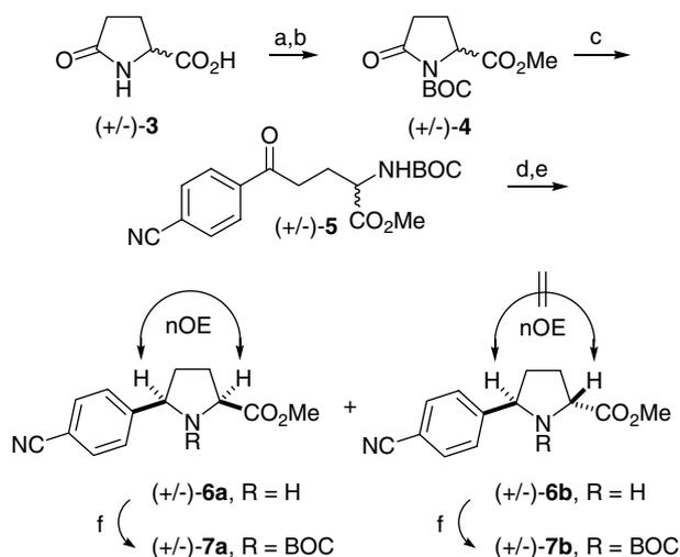
**Scheme 1.** Reagents and conditions: (a) Amberlyst-15, CH<sub>3</sub>OH, 50 °C; (b) Boc<sub>2</sub>O, Et<sub>3</sub>N, DMAP (78%, two steps); (c) 4-cyanophenylmagnesium chloride, -40 °C; (d) TFA, CH<sub>2</sub>Cl<sub>2</sub>; (e) NaBH<sub>3</sub>CN, HCl, CH<sub>3</sub>OH (**6a**: 38%, **6b**: 24%, three steps); (f) Boc<sub>2</sub>O, CH<sub>2</sub>Cl<sub>2</sub> (**7a**: 96%, **7b**: 80%).
