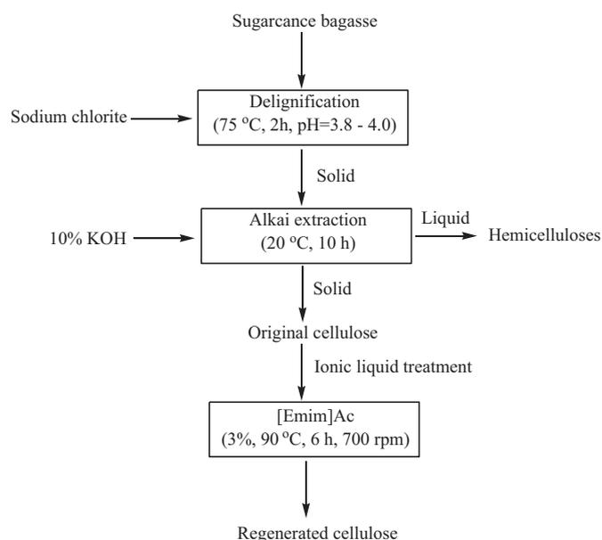
Fig. 1. Schematic illustration of the experimental procedure.
