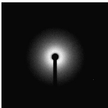
Fig. 1. Wide-angle X-ray diffraction pattern of PEN original fiber.
