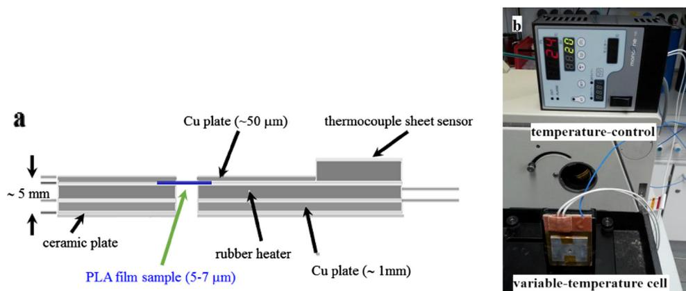
Fig. 1. (a) Schematic illustration of the sample holder and (b) photo of the variable-temperature FT-IR measurement set-up.
