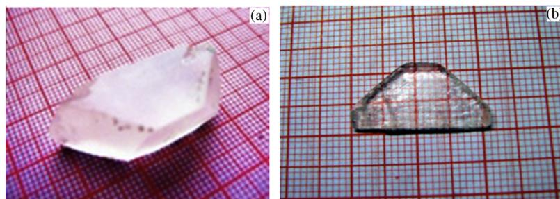
Fig. 1. (a) Bulk  $\text{Eu}^{3+}$  doped LTA crystal. (b) Polished  $\text{Eu}^{3+}$  doped LTA single crystal.
