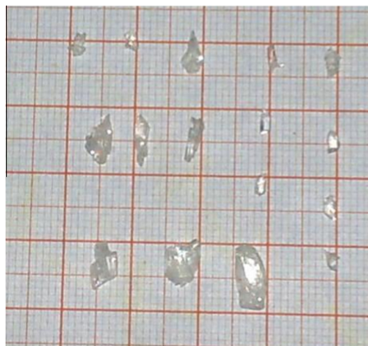
Fig. 1. As-grown single crystals of 2APDHP.
