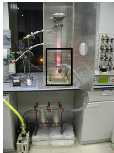
Fig. 1. Picture of the down-stream tubular plasma reactor in the Materials Science Laboratory, IQS.
