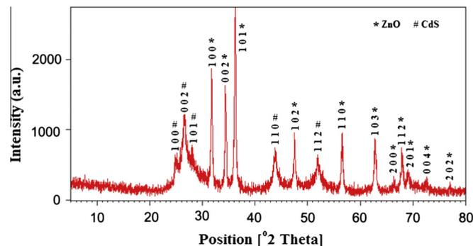
Fig. 1. XRD pattern of  $VO^{2+}$  doped ZnO–CdS composite nanopowder.
