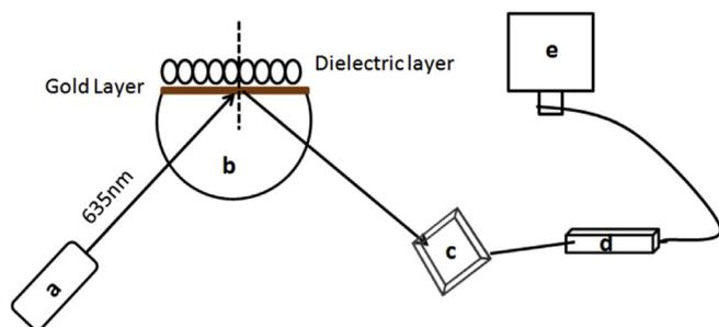
Fig. 1. The schematic of the SPR instrument setup. (a) laser, 635 nm, Newport, (b) semi-cylindrical prism of material BK7, (c) photodiode, OSI-Optoelectronics, (d) Data acquisition card, 12-bit, National Instruments, and (e) computer.
