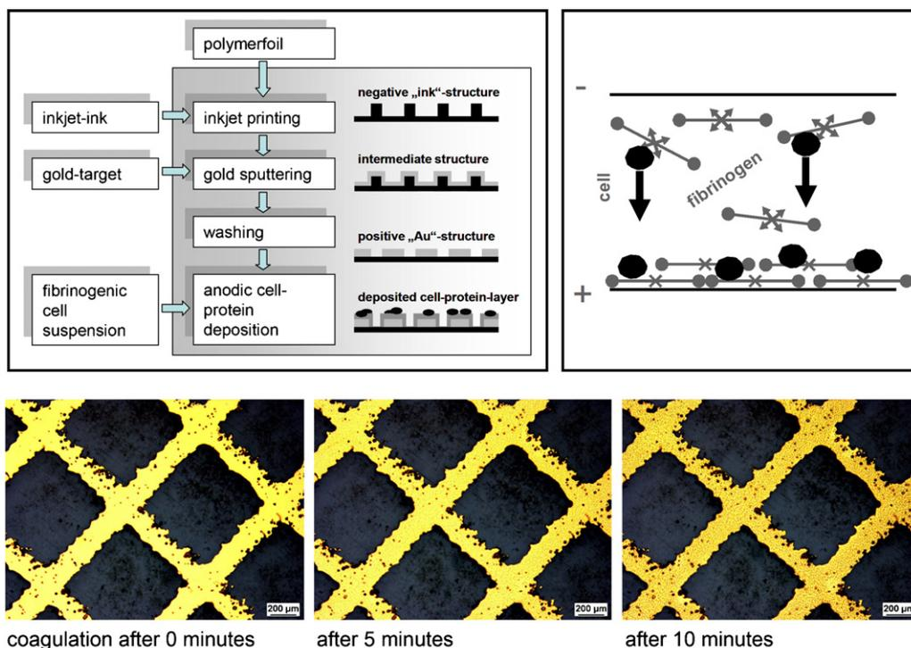
Fig. 1. Processing scheme of the inverse inkjet printing (top) and visual identification of a deposited fibrin-like precipitate on a grid shaped anode (bottom).
