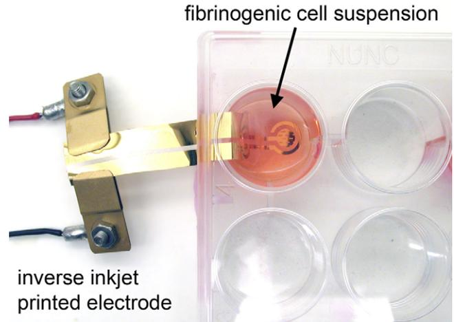
Fig. 2. Sample electrode situated in a 12-well-plate with fibrinogenic cell suspension contacted via gold-coated clamps.
