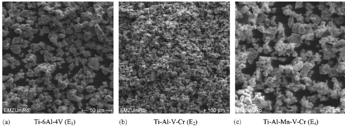
Fig. 1. (a–c) Morphology of the as-milled titanium alloy powders.
