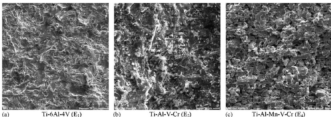
Fig. 2. (a–c) Surface morphology of the FAST/SPS sintered titanium alloys.
