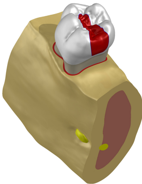
Fig. 1 – Parametric CAD-model (ceramic inlay, adhesive, enamel, dentin, periodontal ligament, cortical bone, cancellous bone) used as a basis for the calculations.
