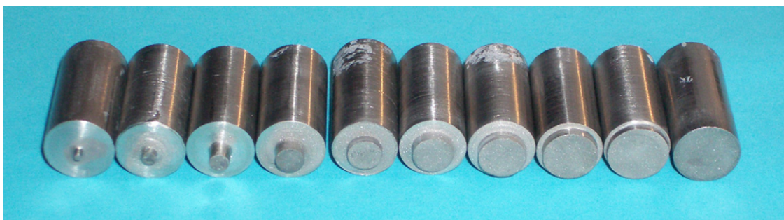
Fig. 2 – Stainless-steel test rods with varying face diameter: 1-10 mm.
