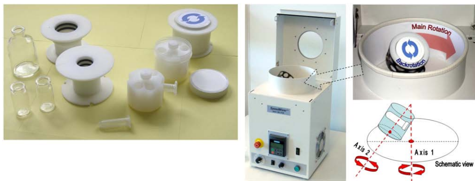
Fig. 1. DAC-principle and -equipment. On the right: Dual asymmetric centrifuge (DAC) with rotation orientations indicated and a schematic drawing of the DAC principle. The drawing shows a vial in the “unusual” horizontal orientation (see Results/Discussion). On the left: suitable glass vials and reaction tubes for DAC as well as the respective vial holders/spindles (left: glass injection vials and vial holders, right: reaction tubes and vial holders for horizontal positioning of the reaction tubes (plus container and spindle)).
