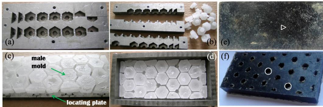
**Fig. 1.** FIHP molds and samples. (a) The mold for the male molds, (b) the prepared molds, (c) the male molds inserted into the locating plate, (d) the spatial relation between the male and female molds, (e) the front of a sample, and (f) the back of a sample. Circles indicate small processing holes.
