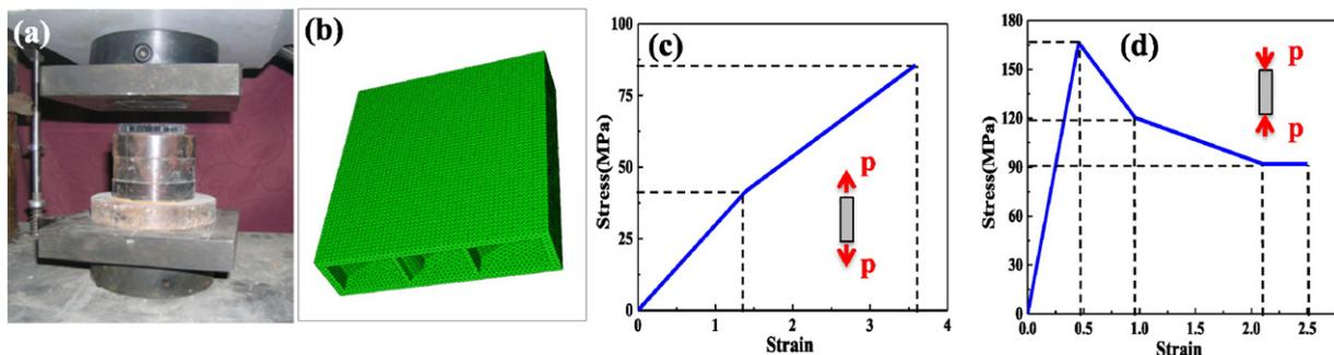
**Fig. 2.** (a) The flatwise compression testing equipment, (b) the meshing of the finite element model, and (c, d) the constitutive relationships used in the model.
