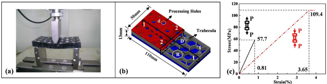
Fig. 1. (a) The test model and pressurization mode, (b) the dimensions of the analytical model of an FIHP, and (c) the constitutive model of the material.
