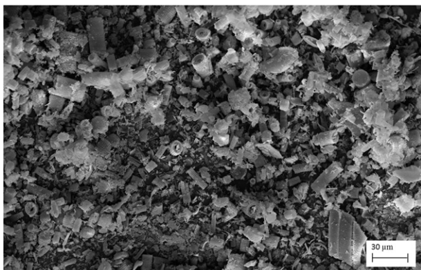
Fig. 2. SEM image of sensor paper surface structure with 1000× magnification and coat weight of 6 g/cm 2 .
