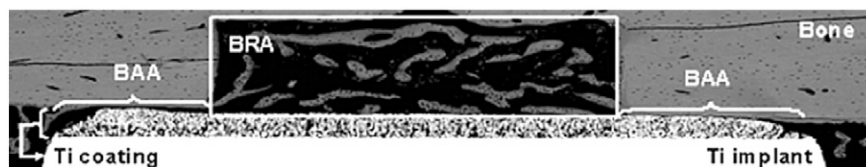
Fig. 1. SEM micrograph of a histological section schematically indicating the regions of interest for histomorphometrical analysis: bone regeneration area (BRA) and bone adaptation area (BAA).
