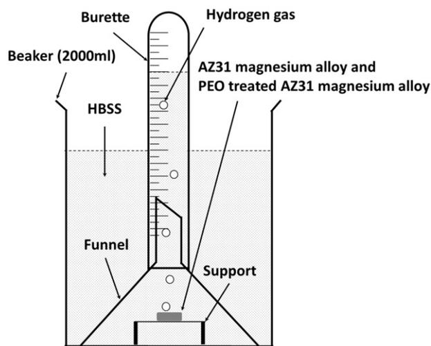
Fig. 1. Schematic illustration for volume measurement of hydrogen evolution during immersion test.
