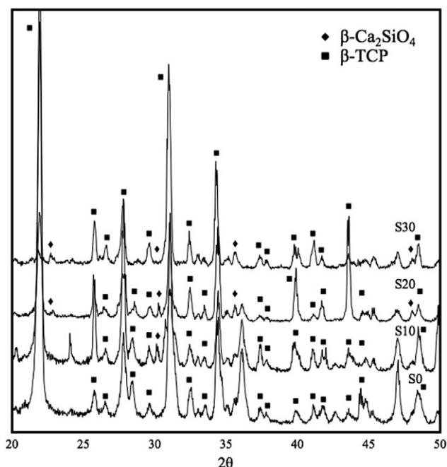
Fig. 2. XRD patterns of cements have different Si-doped ratios after hydration.
