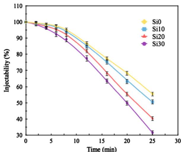
Fig. 1. Injectability of different Si-doped TCP pastes after versus setting time.
