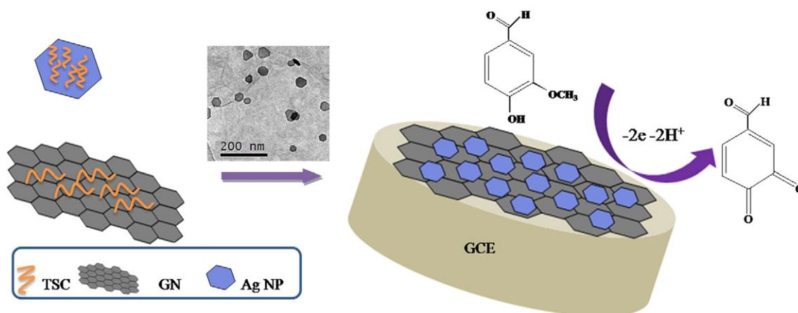
**Scheme 1.** The assembly process of Ag NPs/GN/GCE used in the detection of vanillin.
