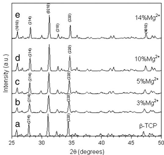
**Fig. 1.** XRD pattern of  $\beta$ -TCMP samples with different  $\text{Mg}^{2+}$  content produced at  $1000^\circ\text{C}$  for 6 h: pure  $\beta$ -TCP, (b) 3 mol%  $\text{Mg}^{2+}$ , (c) 5 mol%  $\text{Mg}^{2+}$ , (d) 10 mol%  $\text{Mg}^{2+}$  and (e) 14 mol%  $\text{Mg}^{2+}$ .
