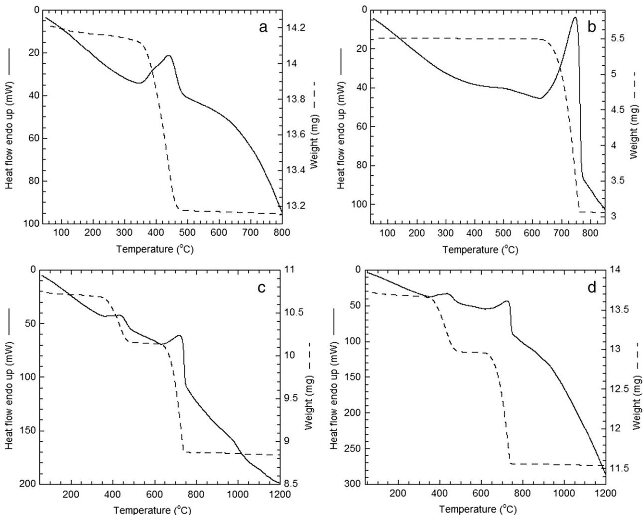
**Fig. 2.** TG/DTA results of different powders: (a) DCPA, (b)  $\text{CaCO}_3$ , (c) mixture of DCPA and  $\text{CaCO}_3$  for synthesis of pure  $\beta$ -TCP, and (d) mixture of DCPA,  $\text{CaCO}_3$  and MgO for synthesis of  $\beta$ -TCMP-5-SS, heated in air at  $10^\circ\text{C}/\text{min}$ .
