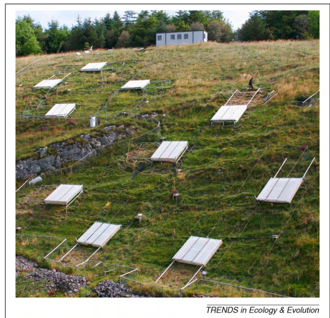
Figure 1. The climate change experiment at Buxton Climate Change Impacts Laboratory situated in calcareous grassland in Derbyshire, UK, is in its 17 th year of continuous climate manipulation, including simulated summer drought imposed with the automated rain shelters seen here. Photo by J. Fridley.
