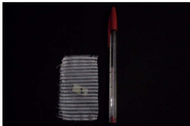
Fig. 1. Preparation of the PU Samples to the biodegradation assay: 1 piece of each sample in small packages.
