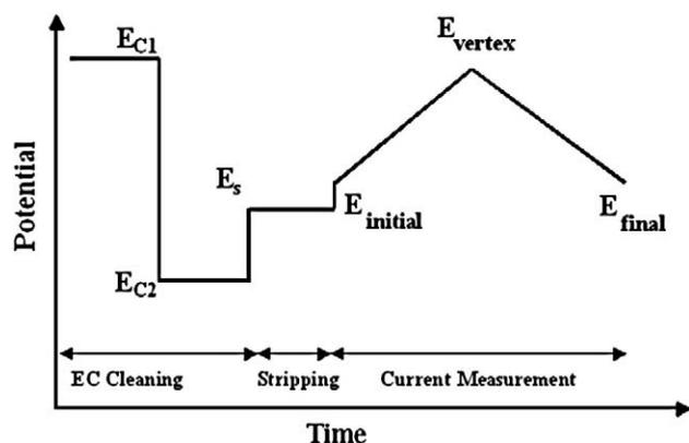
Fig. 1. The schematic of applied potential waveform.
