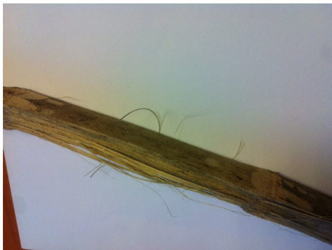
A bamboo stem after splitting and drying and before grinding, classifying and sifting.
