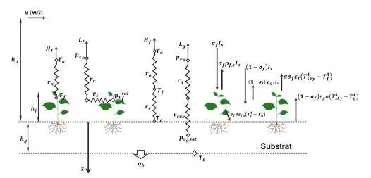
**Fig. 1.** Main modeled heat fluxes on a vegetated envelope module and corresponding heat and vapor transfer resistances. The total vegetated envelope width is  $h_f + h_g$  (foliage and substrate), the backside (building side) temperature is noted  $T_b$  and the transmitted heat flux toward the building  $q_b$ .
