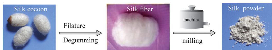
Scheme 1. Schematic illustration of silk fibroin powder fabrication.
