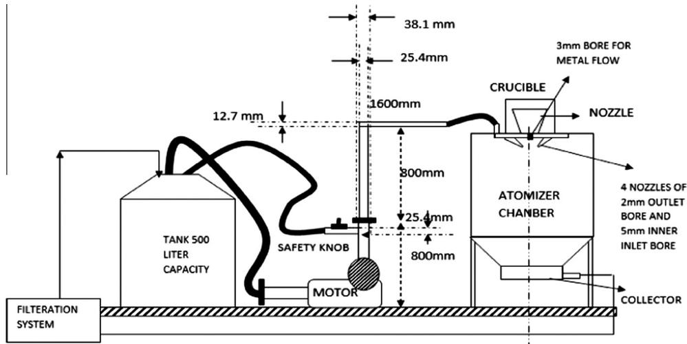
Fig. 1. Schematic sketch of laboratory fabricated water atomizer.
