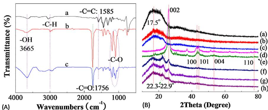
**Fig. 1.** (A) FTIR spectra of (a) the original pristine MWCNTs, (b) PLA with MW of 80000 and (c) MWCNTs/PLA conducting nanocomposites; and (B) XRD patterns of (a–c) PLA with MW: (a) 6000, (b) 50000 and (c) 80000; (d) the original pristine MWCNTs; and (e) MWCNTs/PLA<sub>6000</sub>, (f) MWCNTs/PLA<sub>80000</sub>, (g) MWCNTs-COOH/PLA<sub>80000</sub> and (h) MWCNTs-OH/PLA<sub>80000</sub> conductive nanocomposites.
