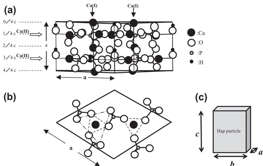
**Fig. 1.** (a) Projection of unit cell of Hap crystal viewed along [110] face, (b) surface structure of the  $c$  crystal surface viewed along [001] face and (c) diagram of sheet-like Hap particle.
