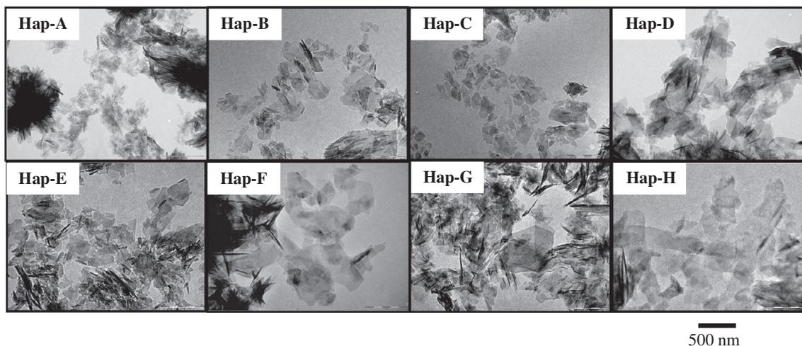
**Fig. 2.** TEM micrographs of the sheet-like Hap particles produced by microreactor (From Ref. [22]).
