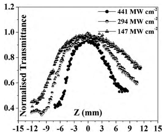
Fig. 3. Open aperture z-scan plot of rf PANI thin films in its pristine form for different laser fluences.
