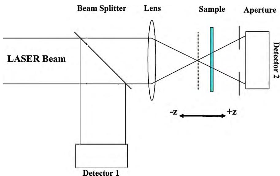
Fig. 2. Open aperture z-scan setup.
