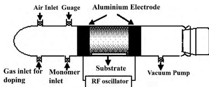
Fig. 1. Setup for rf plasma polymerization.
