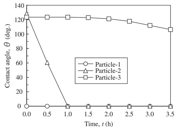
Fig. 1. Time dependences of contact angle for each fluidized particle employed.
