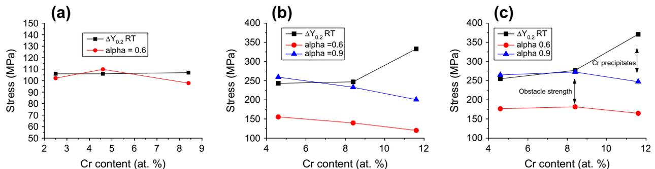
Fig. 1. Hardening measured in Fe–Cr alloys irradiated by neutrons up to (a) 0.06, (b) 0.6 and (c) 1.5 dpa, measured at room temperature (RT) and 300 °C [9]. Prediction of the Orowan dispersed barrier model with loop strength ( $\alpha$ ) taken as 0.6 and 0.9 is also shown. Hardening using the dispersed model was calculated using Eq. (1) and data for loop size and density were reported in Matijasevic and Almazouzi [9].
