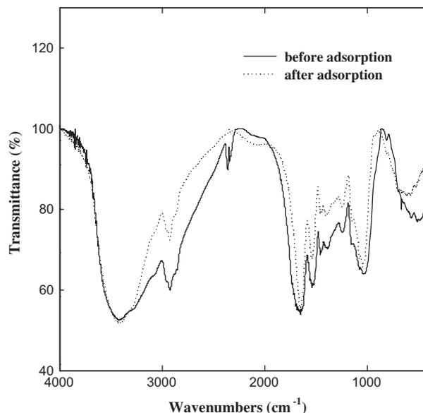
Fig. 1. FT-IR spectra of brewery yeast for before and after the adsorption of RO 16.
