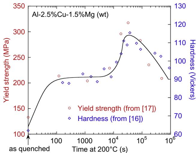
Fig. 1. Evolution of hardness (from Ref. [16]) and yield strength (from Ref. [17]) in an Al–2.5Cu–1.5 Mg (wt.%) alloy as a function of ageing time at 200 °C.
