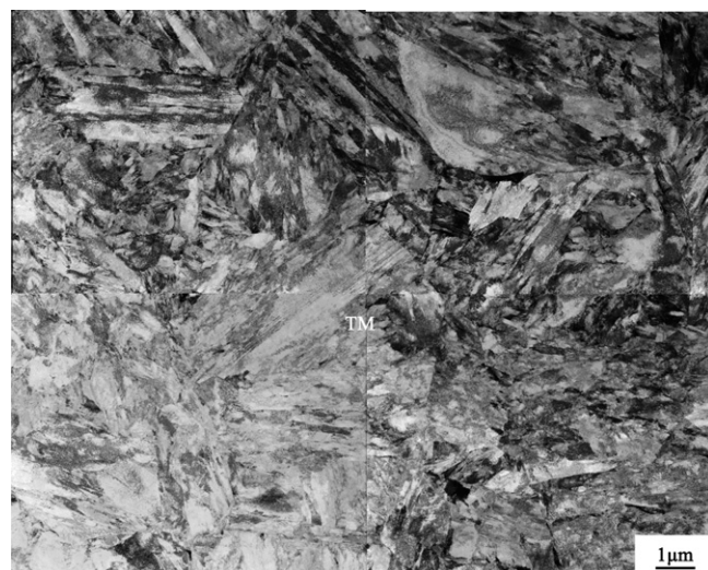
Fig. 1. Microstructure of the 5Mn steel after austenization at 750 °C for 30 min and quenching in oil.
